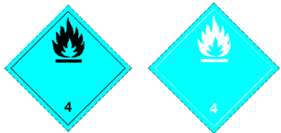
(No. 4.3) Symbol (flame): black or white; Background: blue; Figure "4" in bottom corner
